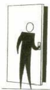
Left Hand Reverse or Right Hand: Hinges on left, opens outward.
