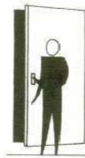
Right Hand Reverse or Left Hand: Hinges on right, opens outward.
