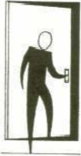
Left Hand: Hinges on left, opens inward.
